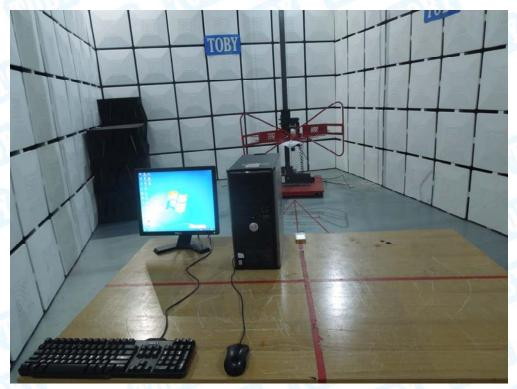
Radiated Emission Test Setup—Below 1G
