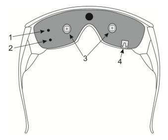
**Picture 1.** 1 – on/off button; 2 – button for choice of work's regimen; 3 – emitters of light; 4 – mini USB-input.
