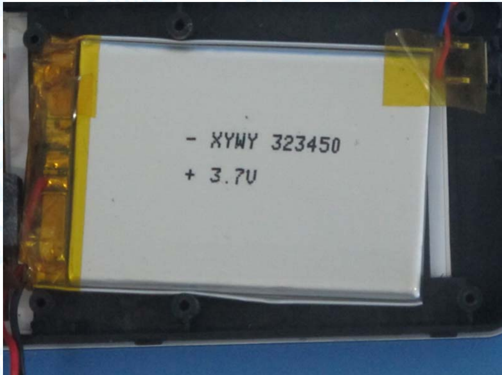
Photo 7 Appearance of Battery
