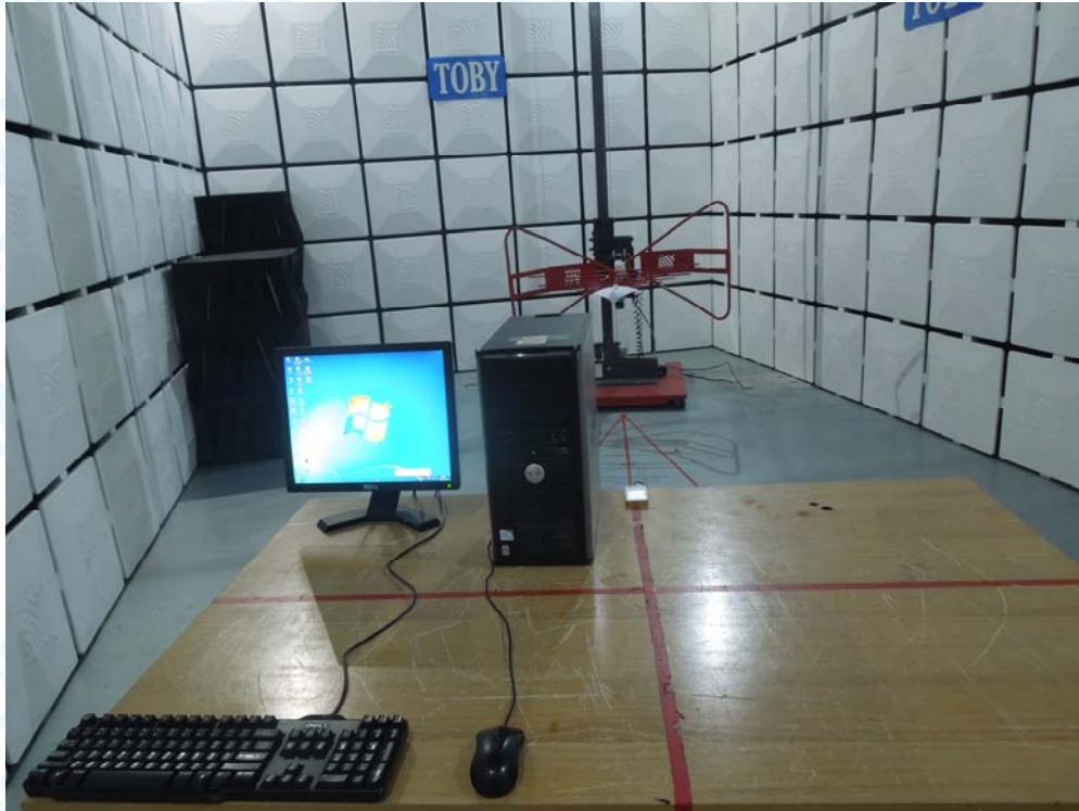
Radiated Emission Test Setup---Below 1G
