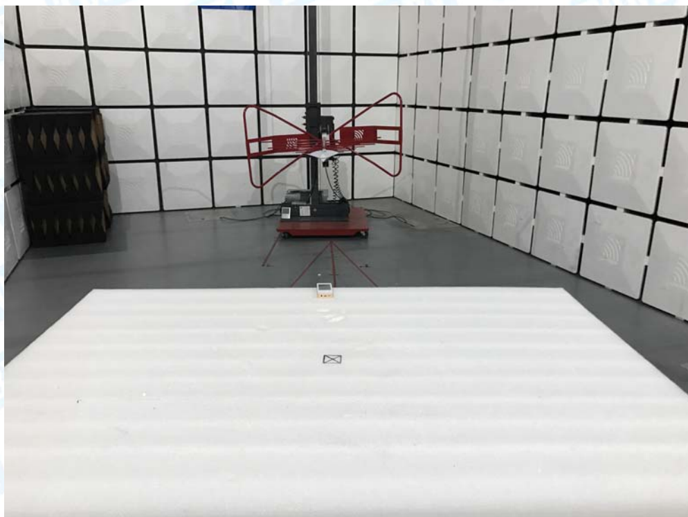
Radiated Emission Test Setup---Below 1G
