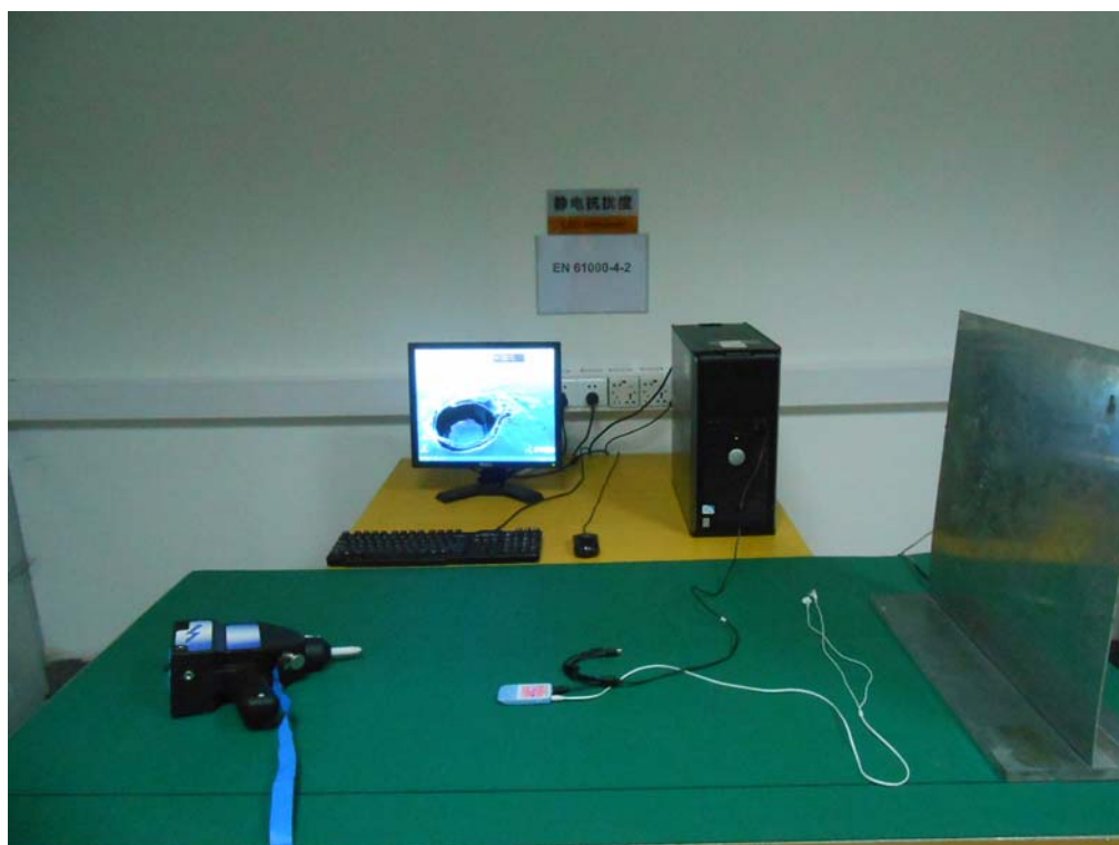
Photo 2 Electrostatic Discharge Test Setup
