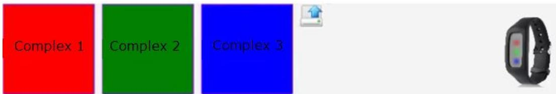
If the complexes were not uploaded to the device, the buttons will be gray and there will be an inscription "Empty". When the complexes are uploaded, the buttons will have a color corresponding to the indication on the device.
